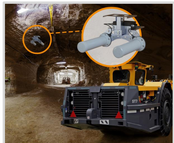
2x HELI-11 antennas mounted on the BRKT-45 for MIMO application
